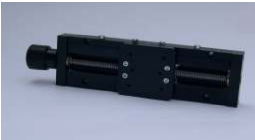
SMMD160-1 Slide with an axis, effective stroke 160 mm, with the follow features: Structure in machined aluminum, trapezoidal brass screw with nut, brass carriage guide and dovetail with gib for the adjustment, handle in knurled aluminum.
